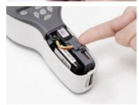
4. Remove the old battery by placing your fingernail underneath the connector's edge and lifting the connector and the battery out of their sockets to disconnect the battery.
