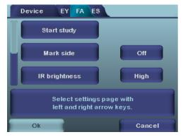
Arrow keys change values in the menu. Active value is indicated with light blue color. Changed values are saved by using left soft key ("Ok") and cancelled by pressing right soft key ("Cancel"). Some values are confirmed by pressing the Middle key.
