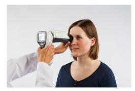
9. Still image is captured by pressing the shutter button all the way down. If half-press capture is enabled, still image can be captured by pressing shutter button halfway down. Taken image is displayed on screen until user clears the image by pressing shutter button, left or right soft key.
