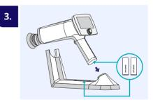
Insert batteries and charge Camera on Charging Station
